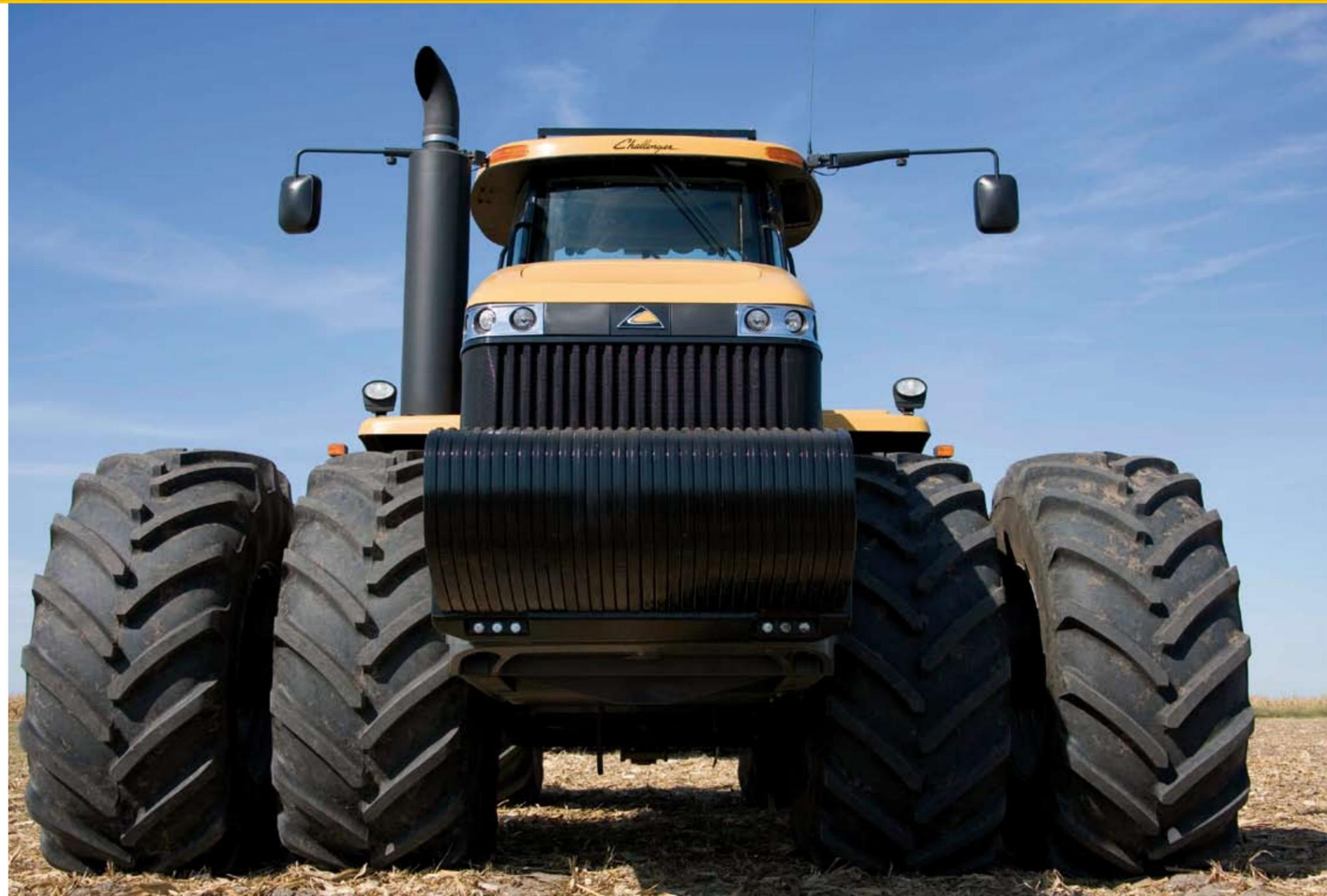
These tractors are powered by Caterpillar ACERT C15 15.2 litre or C18 18.1 litre engines. The Caterpillar Full Powershift transmission, designed specifically for the MT900C, works with the ACERT technology to minimise shift harshness and improve the machine's overall efficiency.
